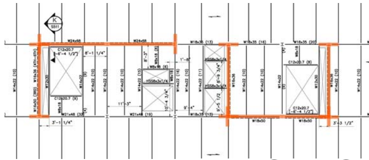
Braced Bay Configuration
